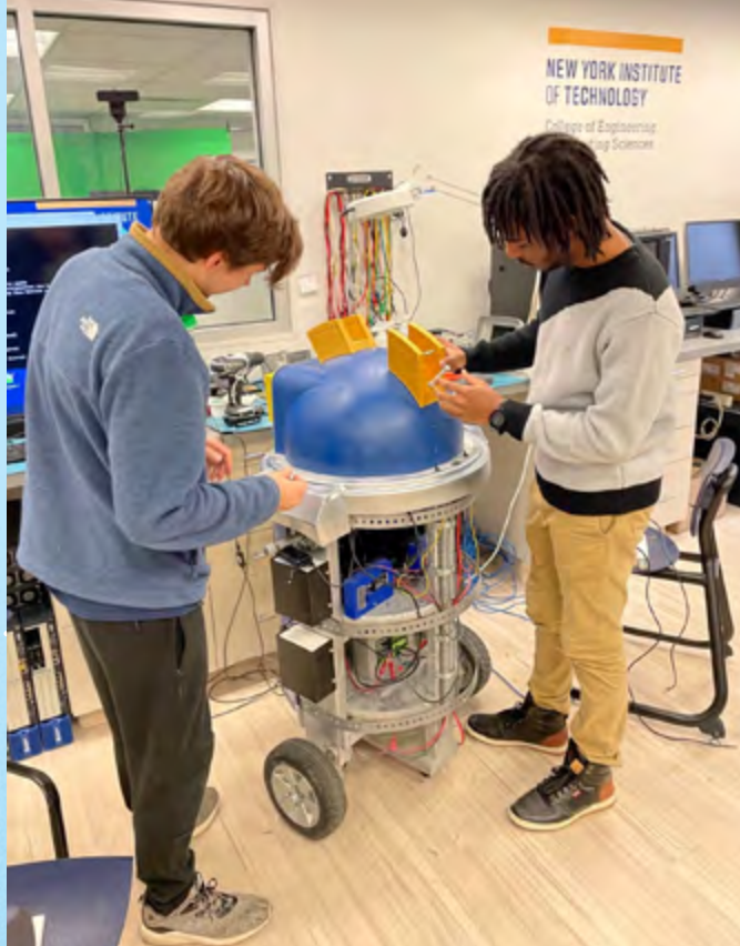
▲ Students configure original mounting brackets for a custom-designed robotic arm that will enable E.R.R.S.E.L.A. to function as a surgical assistant.
